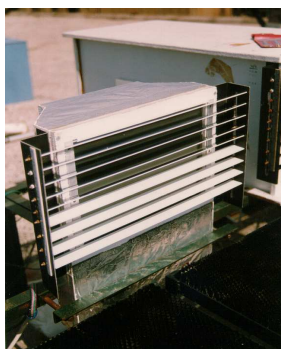
Figura 2-14. Fenestration Radiometer (Pereira, 1992)
